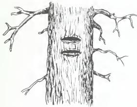
FIGURE 61.—Hack marks on a line tree.
